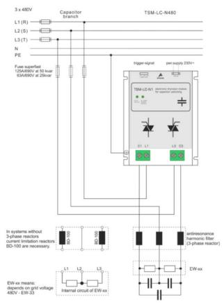
**Pict.2**: Connection diagram, two phase load
