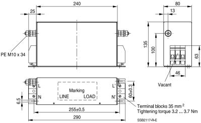
General tolerances according to ISO 2768-cL Dimensions in mm
