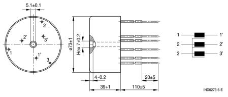
Dimensions in mm Tolerances acc. ISO 2768-c
