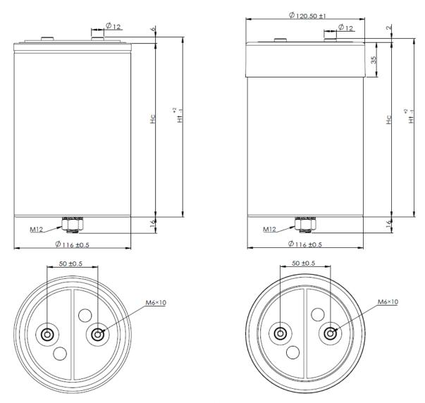
M12 stud on bottom of the aluminum case, nut (DIN 934) and toothed lock washer (DIN 6797) for fixing are standard for all types.
