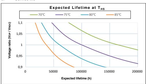
Service life  $t_{LD}$  in hours at different hotspot temperature ( $T_{hs}$ ) and voltage  $V_{RDC}$
